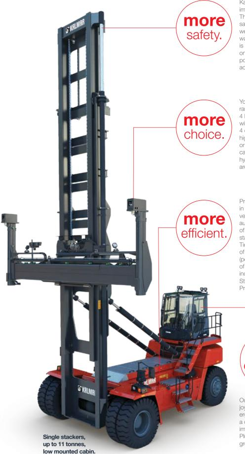
Kalmar smart controls include several important safety functions as standard. The overload protection system offers safety information with the container weight in the main display, including warnings and pop-up messages. There is also a mechanical mast tilt indicator on the tilt cylinder and a transport position striping in the mast for additional driver and operational safety.
